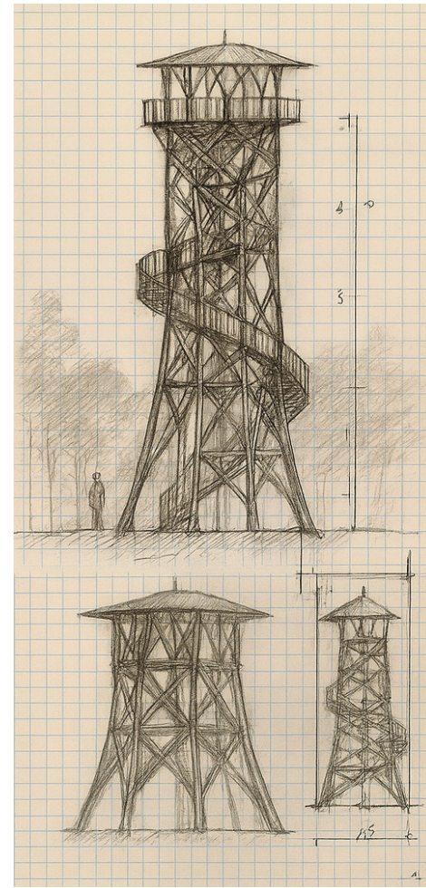
Figure 11 (Left & Right). Tower composition – drawing by Simón Velez with AI evolution by Diana García This image presents a comparative study between an original hand-drawn sketch by architect Simón Vélez and a digitally generated version created by Diana García using artificial intelligence. The hand sketch, drawn on grid paper, outlines the structural concept and spatial proportion of a bamboo observation tower with a spiralling staircase. The AI-generated visualisation expands this idea into a three-dimensional interpretation, emphasising the tower's verticality, its modular logic, and the expressive articulation of diagonal braces. This hybrid approach illustrates how analogue drawings can evolve into spatial models through computational tools, preserving the essence of the original idea while exploring its potential in greater depth. The interaction between the sketched intent and its digital materialisation exemplifies a generative design process that bridges traditional architectural thinking with contemporary design technologies. Reproduced with permission from the architect Simón Vélez.
